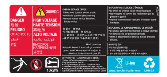
Li-lon batteries have greater risks than the NiMH batteries and therefore additional safety measures need to be followed when handling and storing them. You should consider the following when handling and storing HV batteries:
